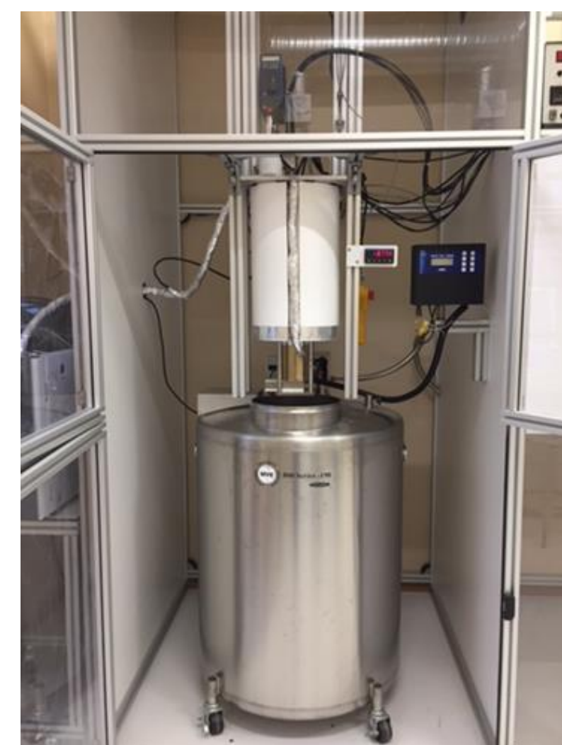
Cryogenic experimental facility for measuring solid-fluid equilibrium (CTP Mines Paris PSL)
